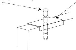
**4.** Attach the Strike Plate as shown on back of door, opposite side of pivot brackets. Use screws pruse screws provided.
