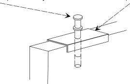
5. Attach the Door Stop (1019) to protrude 1/8" above top of door on back of Pivot Panel.
