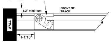
3. Insert top Pivot Pin (1029-1) into factory mounted Pivot Bracket on each door panel.
