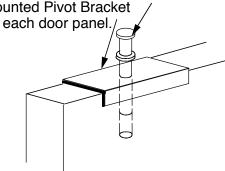
4. Attach the Strike Plate as shown on back of door, opposite side of pivot brackets. Use screws provided.
