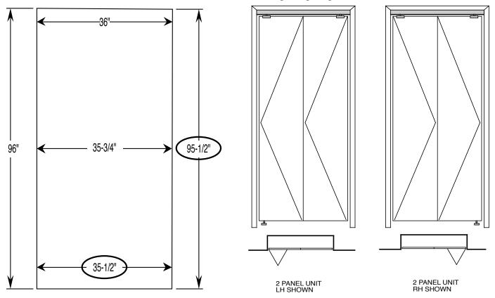
FINISHED OPENING WIDTH TO BE USED FOR THIS CLOSET IS 35-1/2" X 95-1/2".
