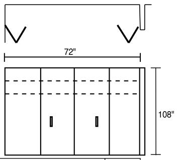
Total cost per opening using primed MAGIGLIDE® system 6'0" X 9'0"
