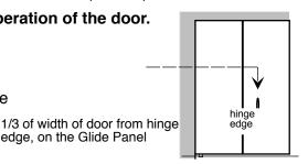
16. On doors with 4 or more panels, mount Door Aligners (1016) on back of panels, as shown in diagram on page 3. Doors of 6'-8" require 2 Aligners placed 4" from bottom of door. 8' tall doors require an additional pair of Aligners located 4' from top or bottom.
